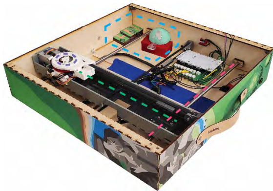
Figure 3: Travelling Forest hardware with x-axis (green), y-axis (pink), orientation theta (purple), and storage area (blue).
